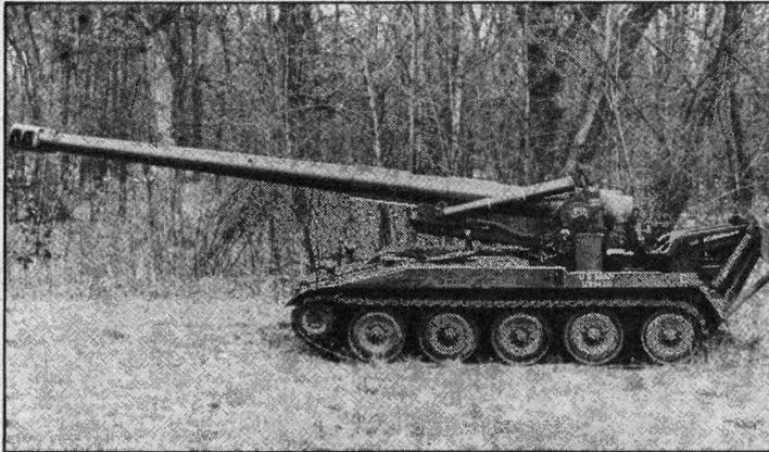
The two faces of the neutron bomb: the M110 howitzer, which fires a rocket-assisted neutron bomb shell for 30 kilometres; (right) and the Lance missile (left).
