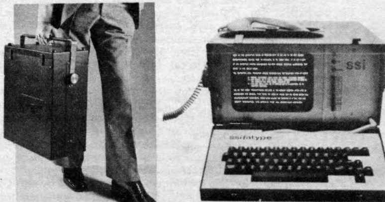
The SSiFATYPE, a commercially available, portable encrypting communications terminal marketed by Security Systems International. At the top is shown a message as the VDU screen reproduces it and, below, its encoded format
